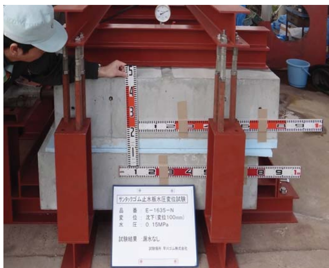
沈下量100mm/耐水圧0.15MPa
