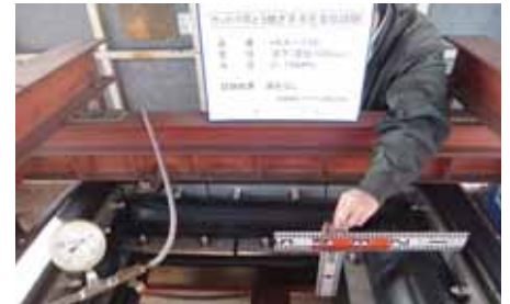
沈下量100mm/耐水圧0.15MPa
