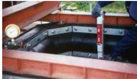
伸び量100mm/耐水圧0.15MPa
