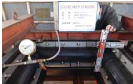
伸び量100mm/耐水圧0.15MPa
