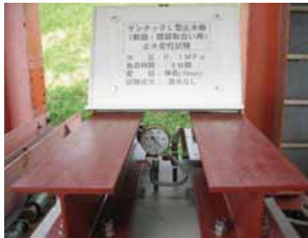
伸び量30mm/耐水圧0.1 MPa
